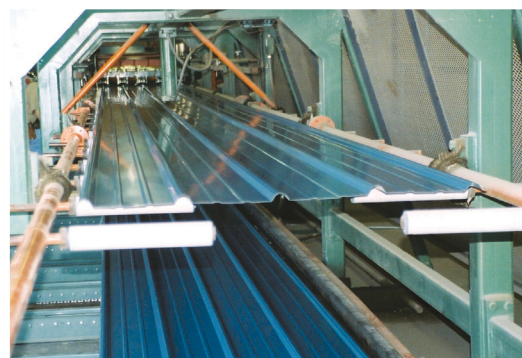
Wall and roof steel roll former up to 48' length
